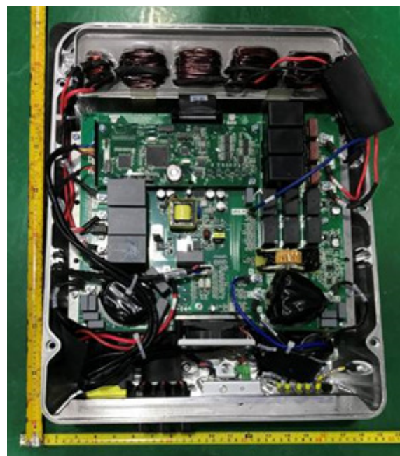
Figure 4 Converter Internal view for model: OG-12K-DM, OG-15K-DM
